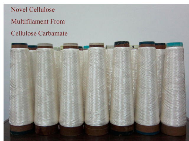
Figure 1. Photograph of the novel RC multifilament produced by a pilot machine from cellulose carbamate.
